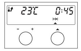
■ Enter the duration in Hours:Minutes by turning the (-/+) input dial (left hand dial).
